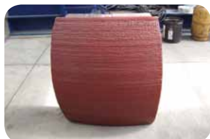
Figure 4 (top left): castings supplied before surfacing alloy
