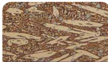
Figure 3: the structure of an Fe-Cr-Nb-C alloy
